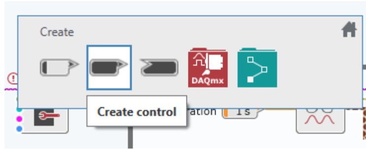
Figure 6-13 Create controls, constants, and indicators by right-clicking on the terminals of a block diagram element.
