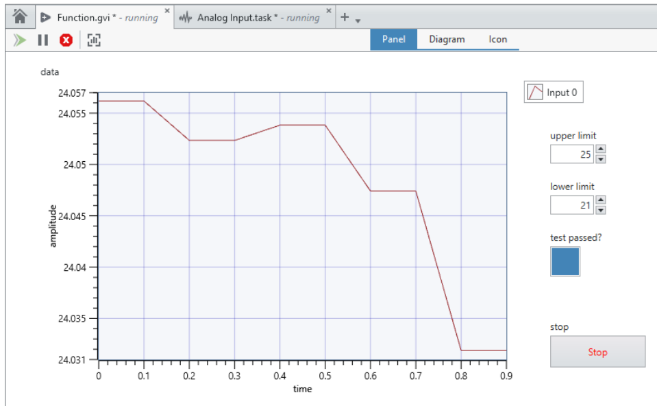
Figure 3-24: The Front Panel will allow the user to define the upper and lower limits of the temperature range.
