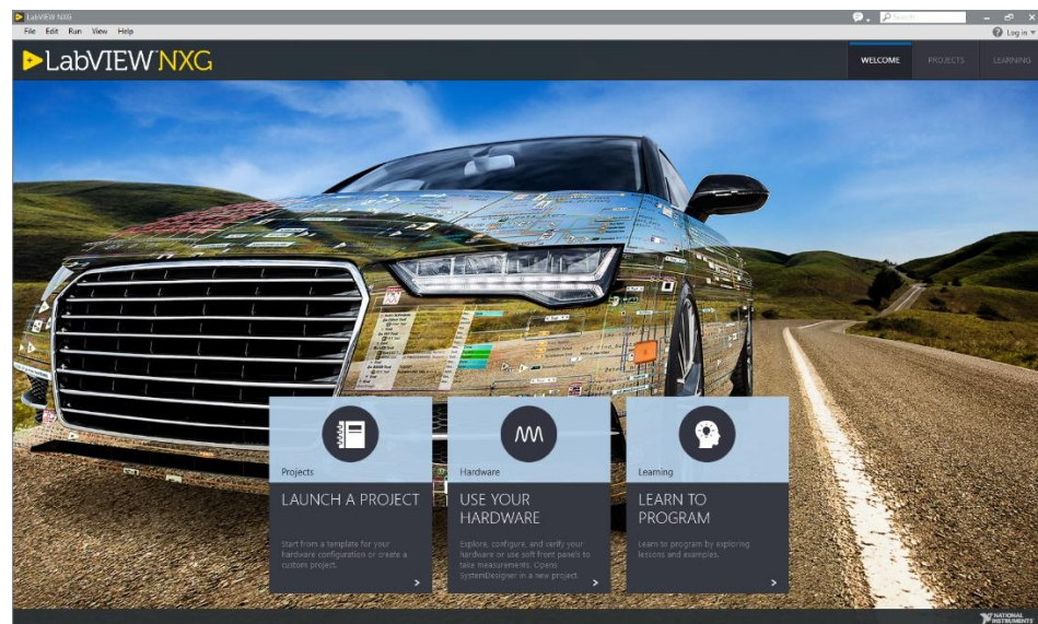
Figure 5-3: Click Use Your Hardware to configure a simple measurement for checking signal connectivity.
