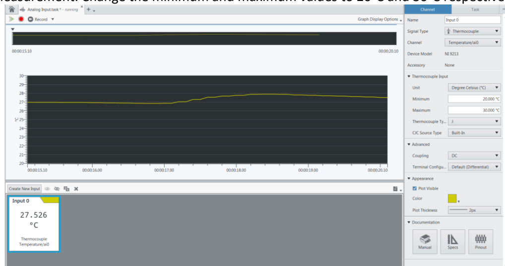
Figure 1-8: After modifying the channel settings in the Configuration Pane, you will be able to view your temperature.
