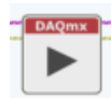
Figure 7-27 DAQmx start commits the task configuration and transitions it into the running state to begin acquisition or generation.
