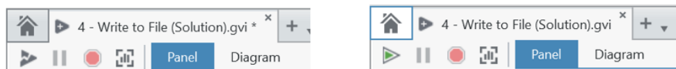
Figure 3-5: A broken run arrow (left) indicates that there is an error compiling this application.
